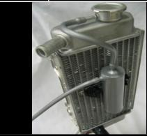
5. Make sure the canister is fastened securely to the radiator and that all hoses are attached correctly before use.
